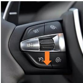
**Rocker down:** Exhaust flaps are kept closed up to a predefined speed which can be set via configuration software
