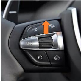
**Rocker up:** Exhaust flaps are opened and kept open over the entire speed range
