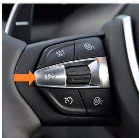
**RES button:** Exhaust flap function is reset to "Series" mode.
